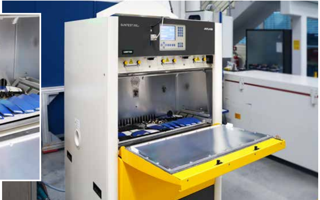
The weathering chamber is also suitable for 3-dimensional test specimens or cut-outs of excessively large test specimens.
