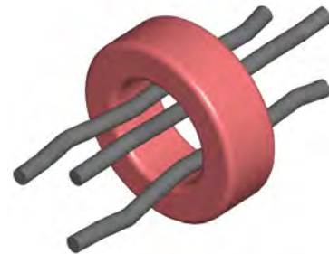
Toroidal core for motor cable
