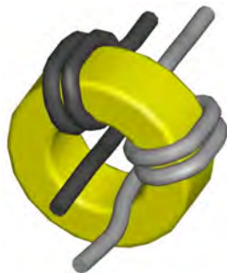
Toroidal core in BR09-1 and BR11-A
