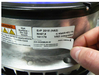
Sticking the AM-MODBUS-W inside label on the ECblue housing.
